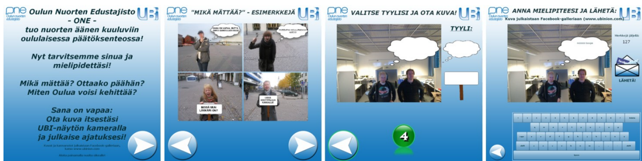
Figure 4. The screens of Ubinion application. From left: initial instruction screen, example opinions and feedback, webcam image and choice between "speech bubble" or "protest sign" as the augmenting element, and a screen with virtual keyboard to enter text in the chosen graphical element and a submit button.
